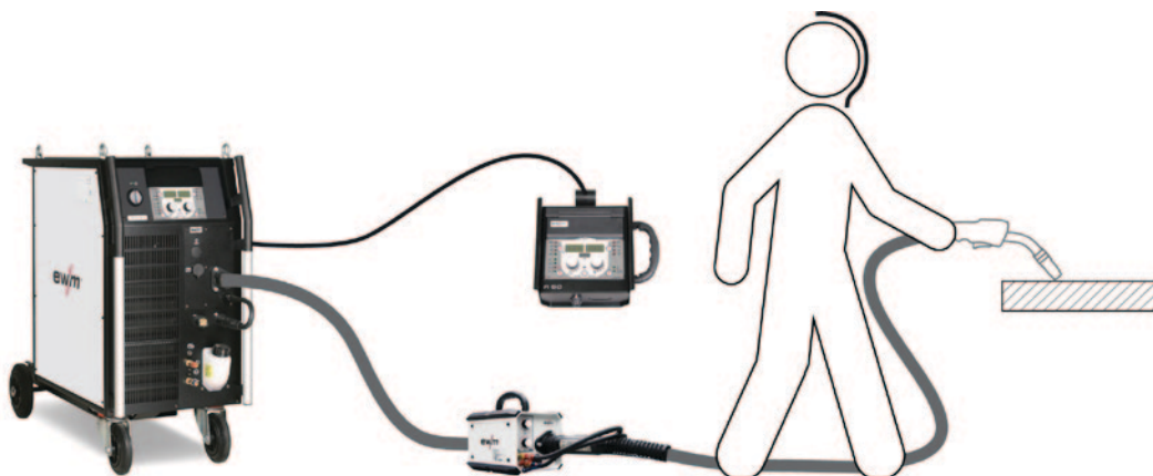
R50 7POL as a second remote control with compact welding machine and miniDrive
