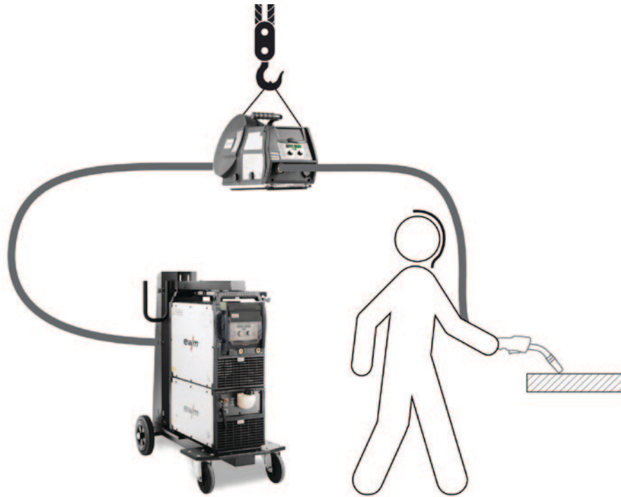
R50 7POL plugged into the welding machine as a second control
